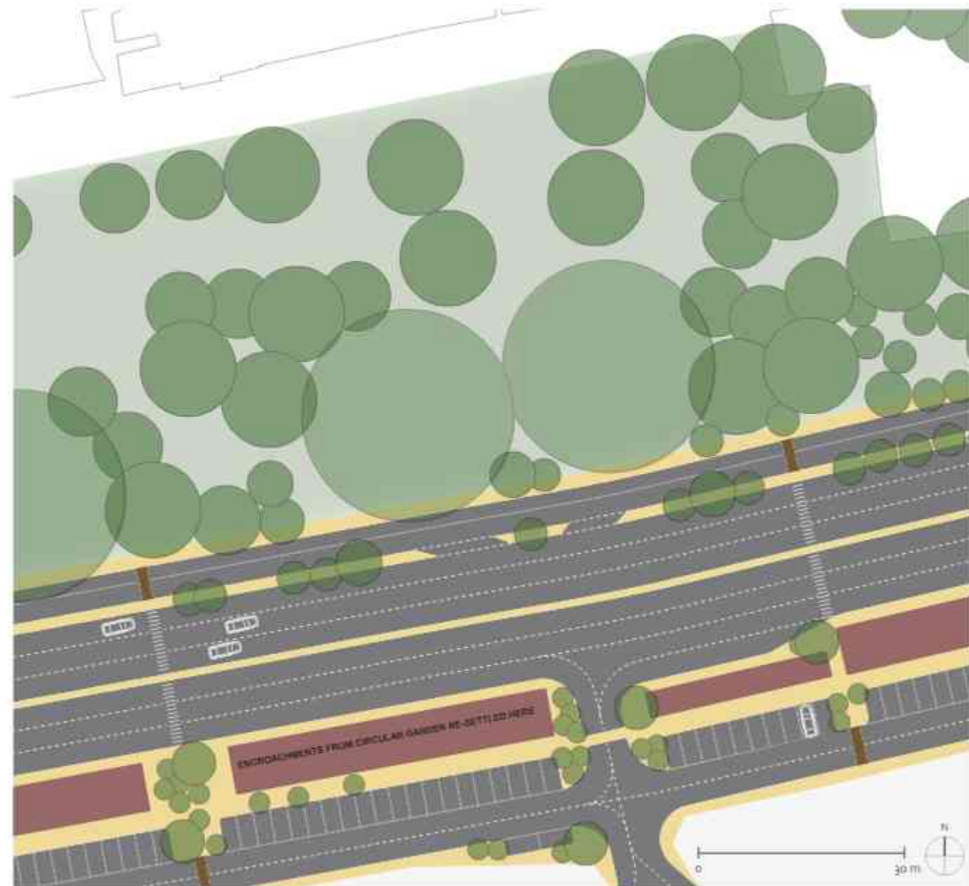
FIG. 62 PROPOSED RE-DESIGN OF THE RIGHT OF WAY ALONG SOUTH-EAST CIRCULAR ROAD. DETAIL OF CIRCULAR GARDEN AFTER REMOVAL OF ENCROACHMENT. OPPOSITE PAGE, SECTION THROUGH THIS PART OF CIRCULAR ROAD
