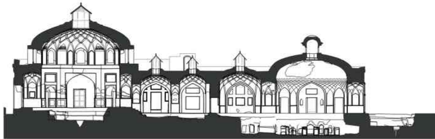
Shahi Hammam Section AA (After Excavations)
