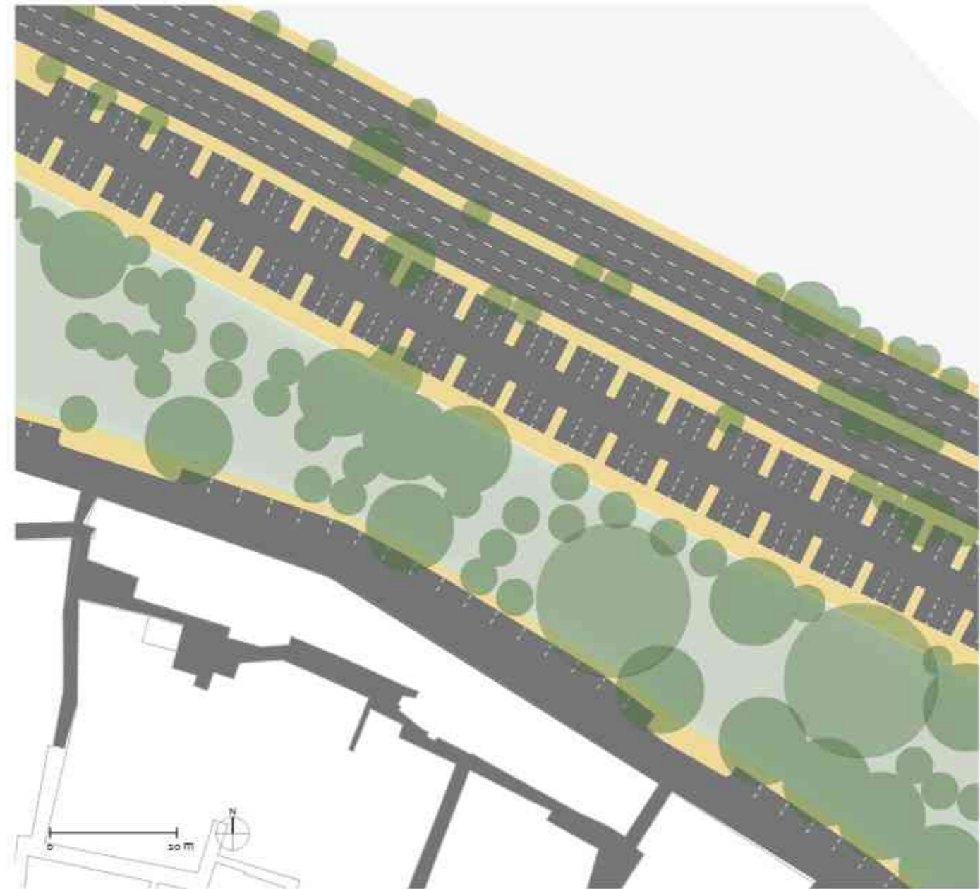
FIG. 53 DETAIL OF PROPOSED SERVICE LANE & PARKING AREA NEAR SHARIF HOSPITAL NORTH CIRCULAR ROAD
