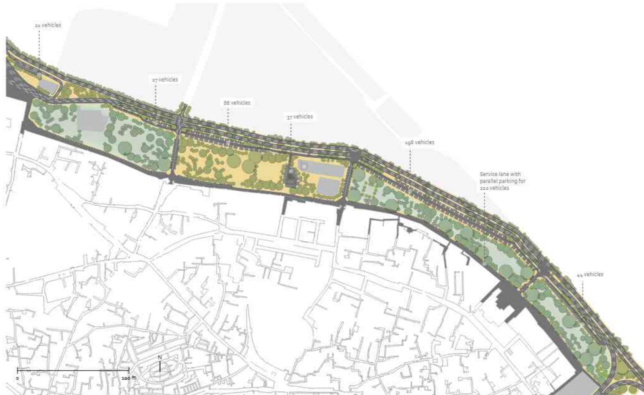
FIG. 52 TRAFFIC ENGINEERING AND RE-DESIGN OF NORTH CIRCULAR ROAD, SHOWING LAYOUT OF PARKING ZONES AN ENLARGED DETAIL IS SHOWN ON THE OPPOSITE PAGE
