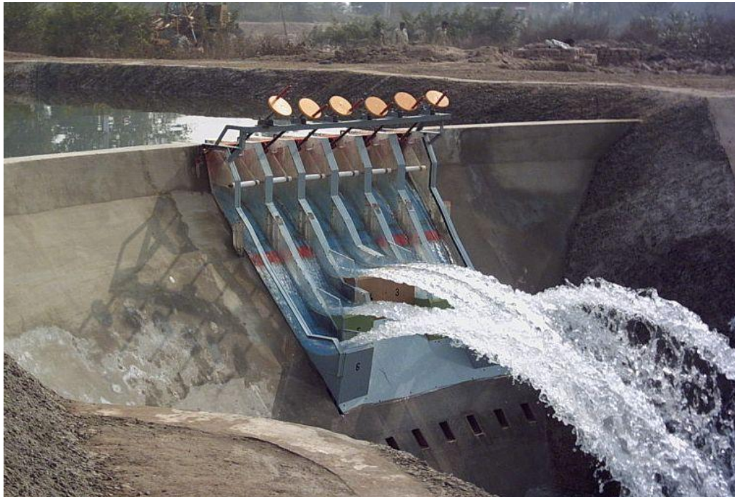
EXHIBIT 10: Downstream View of Dasu Dam Model
